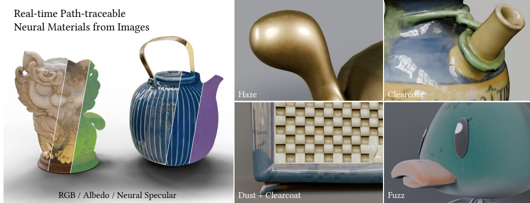
Figure 1: NeuMatEx extracts Neural Materials , a richer material representation that goes beyond PBR, from multi-view images. NeuMatEx decomposes a diffuse lobe and neural specular lobes to model complex material-light interactions such as haze , dust , clearcoat , fuzz , scatter , and their mixtures. The extracted neural materials support real-time path tracing on a commodity GPU.
